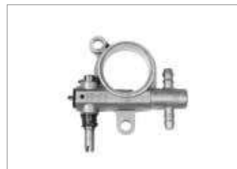
Adjustable aluminium oil pump: facilitates the operator's job by allowing the oil feed to be adjusted to suit the workload on the machine and the bar/chain combination. Zero oil flow with the engine at idling speed ensures lower consumption and reduced environmental impact.
