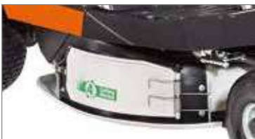
"4-cutting device": versatile cutting system that includes mulching, collection and side discharge as standard, with deflector for rear discharge.
