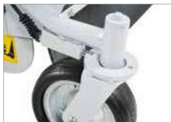
Pivoting front wheels, lockable from the driving position (model 100 , 100 TR ).
