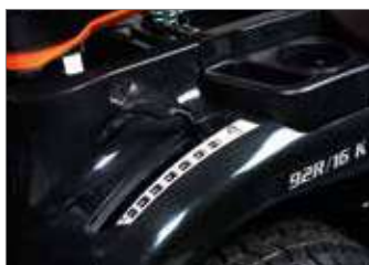
Practical cutting height adjustment with a conveniently positioned lever, with a graduated scale to show the cutting height at a glance.
