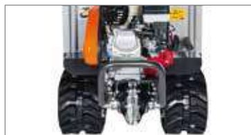
Rear metal guard to maximize operator safety.
