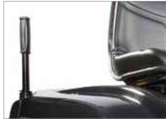
The telescopic bag emptying lever positioned within easy reach of the driver's seat allows the operator to tip and empty the full bag effortlessly and without twisting the body.
