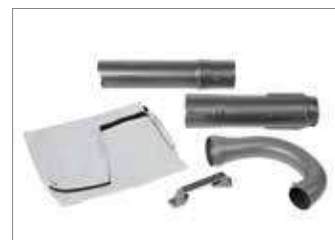
Vacuum cleaner kit (optional): comprising a side handgrip with integrated anti-shock system, a suction tube, an elbow tube and a collection bag, it transforms the blower into a vacuum cleaner for collecting leaves, grass and small pruning debris.
